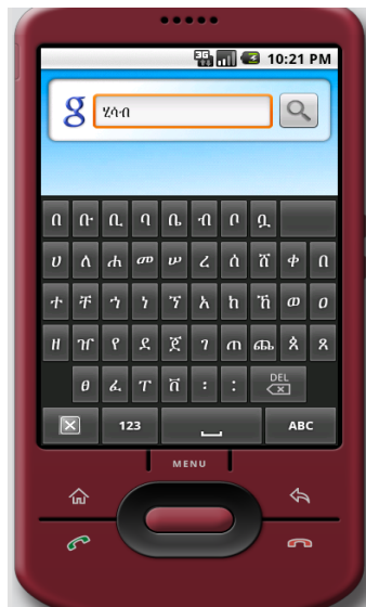
Figure 5.2: The input of the letter “ሰ” after tapping the button for “ሰ”.
