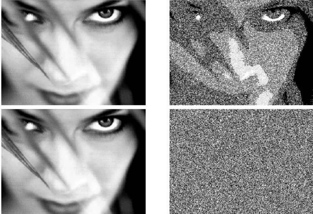
Figure 1: LSB plane example using two images. Upper left image is the original photograph, and upper right is its least significant bit plane with 0 set to black and 1 set to white. The lower left image is a message embedding with S-Tools and the lower right is its LSB plane. Images from [11].
