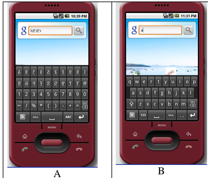
Figure 5.3: (A)-The panel for Ethiopian and Amharic numerals and Mathematical symbols; (B)- the Virtual QWERTY keyboard.
