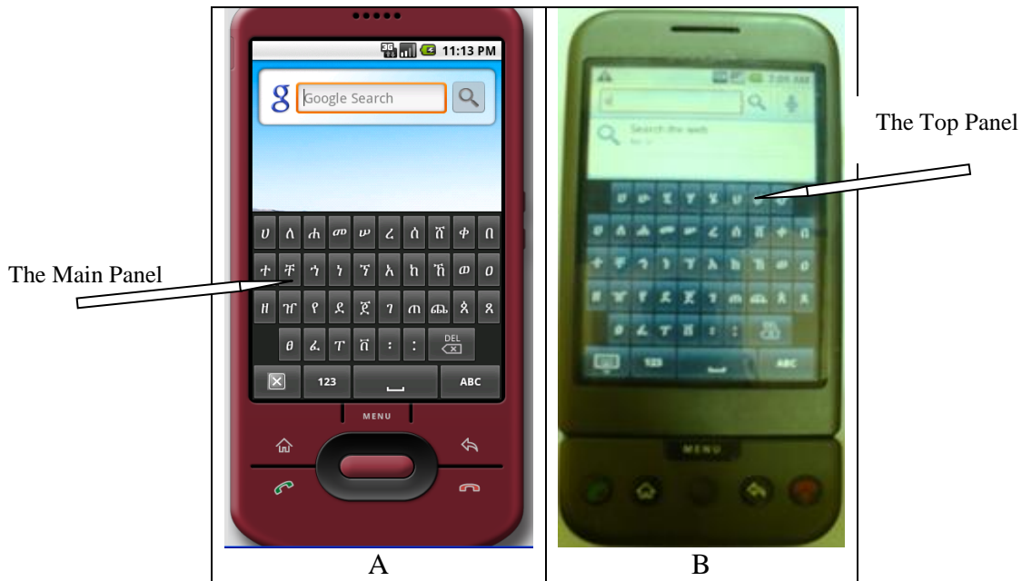
Figure 5.1 VEK on Android Emulator (A) and on the Android based HTC G1 smart phone (B).
